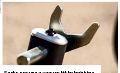
Forks ensure a secure fit to bobbins
